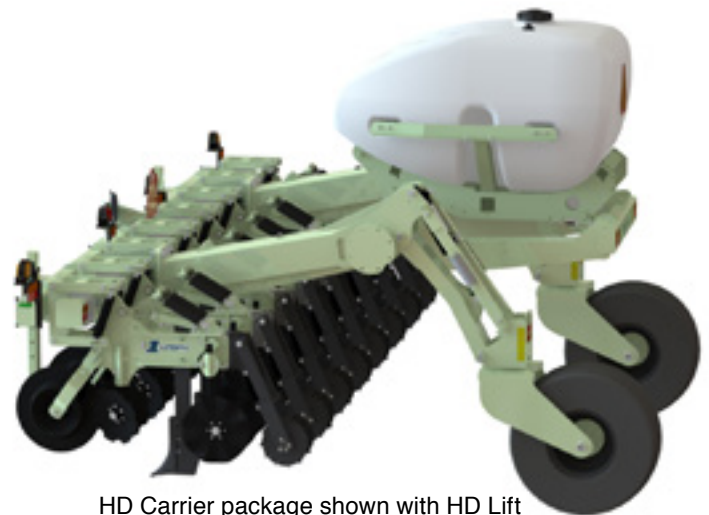
HD Carrier package shown with HD Lift Assist Wheels and 8 row 1tRIPr.
