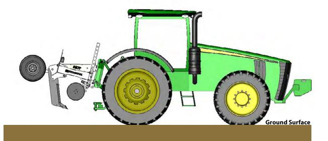
**TRANSPORT POSITION.** During transport, the tractor 3-point hitch should be in the fully raised position
