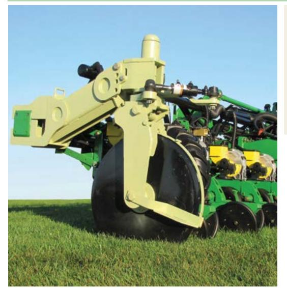
Based on the same operating principles as the Tracker IV, the Shadow Tracker includes a single cylinder and blade that can be mounted in combinations of up to 4-blade systems depending on the size of the implement and field terrain.
